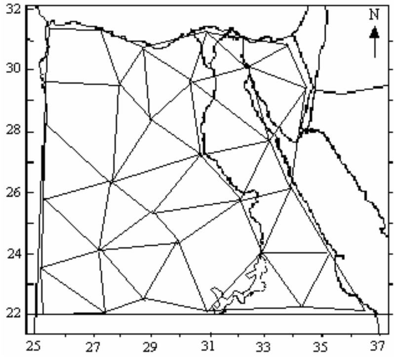
Figure 1: The High Accuracy GPS Reference Network (Order A)
